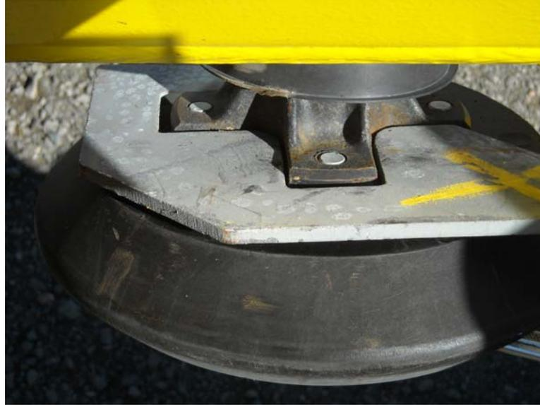
The conveyor wheel replacement tool is used to facilitate conveyor wheel replacement. Its use is shown above and fully detailed in Technical Brief TB 091120-Rev. 0.
