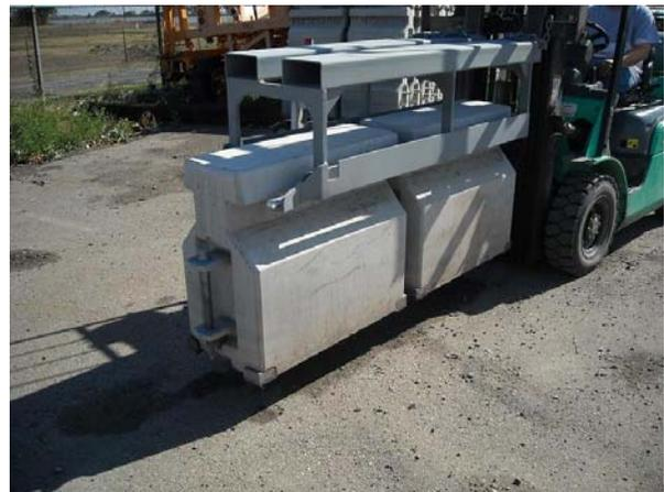
Double lifting device is a fork lift attachment used to transport a pair of QMB. They are the most efficient tool for setting the wall, loading and unloading barriers, and stacking QMB in the storage are.
