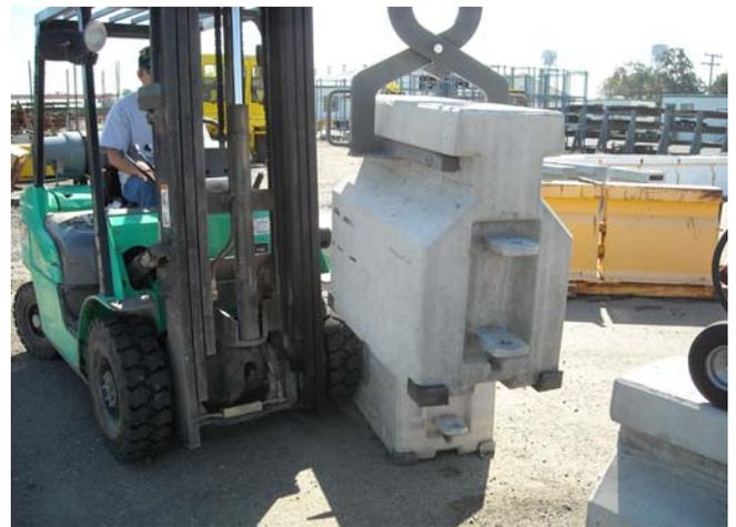
Barrier lifting tongs are for the installation and removal of 1 to 2 concrete barriers. This tool is mainly used to replace a damaged barrier in the wall. They have been used for setting a long wall, but are much slower than using a Forklift Double Lifting device.[see next page] When lifting 2 barriers at the same time, the center pin must be installed and e-clipped.
