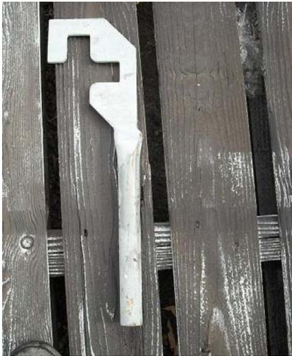
To replace the conveyor wheel, place the hub wrench, shown in figure 2, on back of the hub to keep hub from spinning, as shown in figure 3 below. Then using a  $\frac{3}{4}$  inch or 19mm wrench or socket remove the four bolts and the back-up plate (B880601) as shown in figure 4, below.
