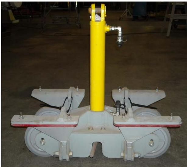
Hydraulic pin pusher used to drive pins through the hinges.
