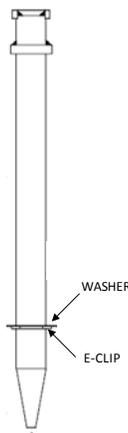
Figure 3 E-Clip installation detail
