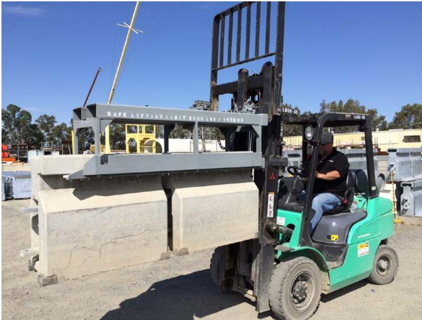
Figure 1 Double handling device
