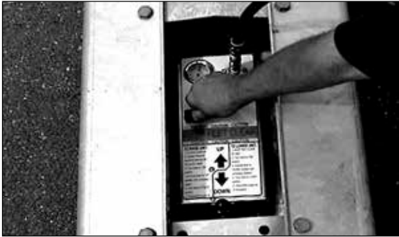
Figure 6. Move the selector handle from the LOCK position to the ON position
