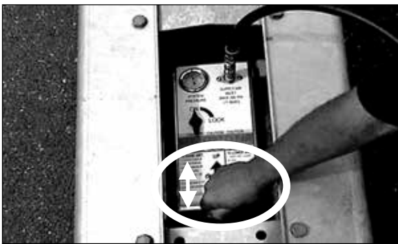
Figure 7. Activate the jack by moving the direction handle located on the end of the panel in the UP or DOWN position.
