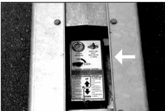
Figure 8. Before removing the air supply from the Supply Air Inlet, move the selector the LOCK position.
