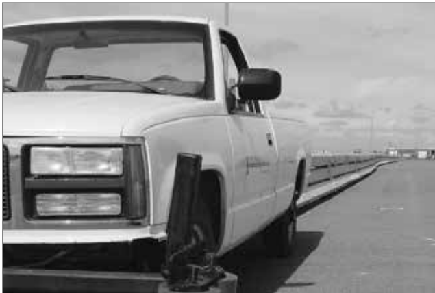
Figure 22. Pull the barrier straight or at an angle. For an angled move, all of the steering wheels (using the tiller handle) must be positioned in the desired direction. Always use caution when towing large sections of barrier.
