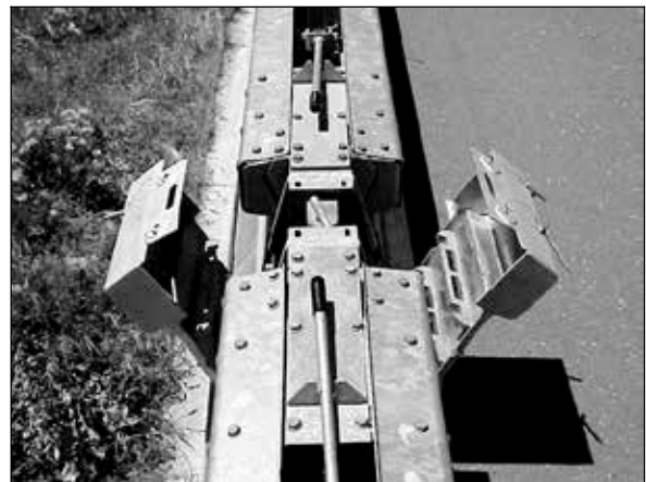
Figure 15: The hinge covers will stay upright and opened after the cover is installed as instructed above.
