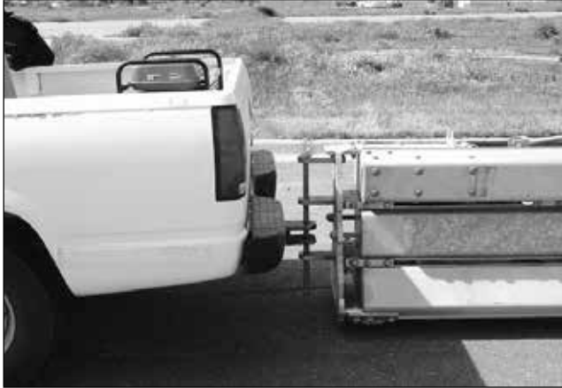
Figure 21. Attach the length of link barrier to a truck using a chain or a hinge pin as show above.
