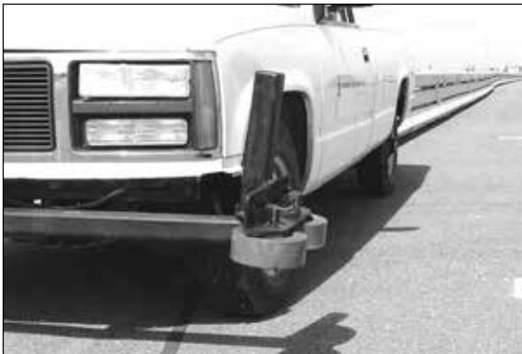
Figure 17. The push rollers move the barrier sections without causing damage.
