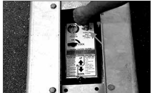
Figure 5. Connect the air supply hose to the Supply Air Inlet fitting located on the top (or on some models the end) of the Control Panel. Adjust the Supply Air Inlet regulator until you see approximately 120 psi on the System Pressure gauge.
