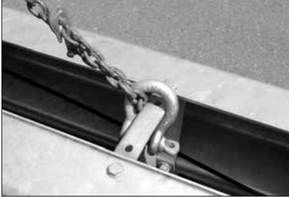
Figure 1. Use the holes located in the tops of the inboard diaphragms as two lifting points. Lift with a hook or clevis and a suitable cable or chain. Follow OSHA guidelines for safe forklift operation.
